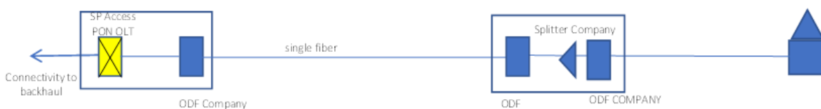
Figure 3: PON Solution with equipment in Central POP
