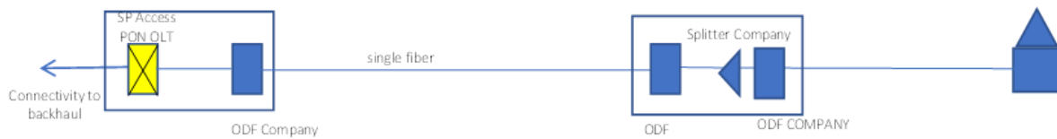
Figure 3: PON Solution with equipment in Central POP
